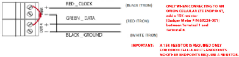
Figure 41: ORION Cellular LTE endpoint connection with resistor
