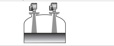
Figure 3-3: There is no maximum limit to the number of devices that can be operated in the same tank
