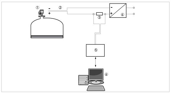
Figure 4-4: Point-to-point connection (non-Ex)
