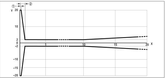
Figure 2-5: DN40 (1½<sup>--</sup>) Lens antenna: measuring accuracy (graph of measuring accuracy in mm against measuring distance in m)
