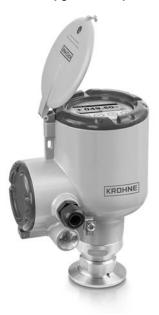
This 80 GHz FMCW radar transmitter for hygienic liquid applications in the pharmaceutical, food and beverage industries is CIP-SIP suitable and offers a large choice of hygienic process connections: Tri-Clamp®, Tuchenhagen VARIVENT®, SMS, DIN 11851, DIN 11864-1 Form A, NEUMO BioControl®.
