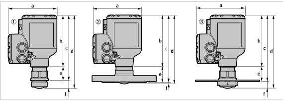
Figure 2-17: DN40 / 11/2" Lens antenna versions
