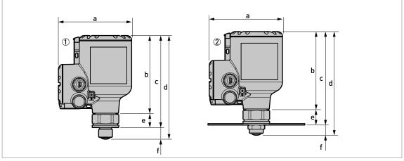
Figure 2-15: DN20 / ¾" Lens antenna versions
