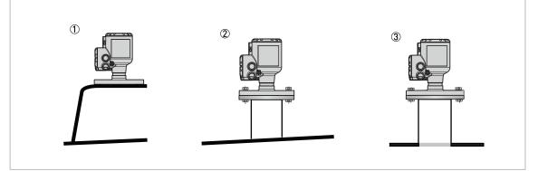
Figure 3-8: Device installation on tanks made of a non-conductive material
