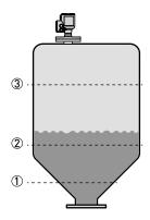
A strapping table function is available in the configuration menu for volume or mass measurement. Up to 50 volume (mass) values can be related to level values. For example: Level ① = 2 m / Volume ① = e.g. 0.7 m<sup>3</sup> Level ② = 10 m / Volume ② = e.g. 5 m<sup>3</sup> Level ③ = 20 m / Volume ③ = e.g. 17 m<sup>3</sup>
