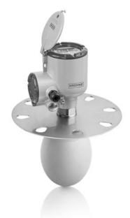
By combining high signal dynamics and FMCW radar technology, this market-entry 24 GHz radar device measures accurately and reliably the level of solids like stone, plastic granulates or coffee beans. No need for expensive antenna aiming kits or purging systems; the proven Drop antenna design minimizes scaling and is not affected by the angle of repose.
