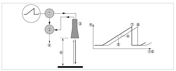
Figure 1-1: Measuring principle of FMCW radar
