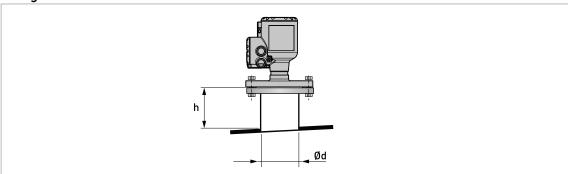
Figure 3-6: Flange connections
