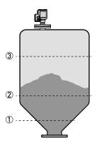
A strapping table function is available in the configuration menu for volume or mass measurement. Up to 50 mass (volume) values can be related to level values. For example:
