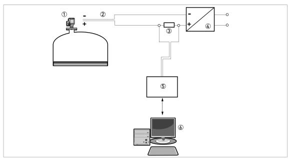
Figure 4-4: Point-to-point connection (non-Ex)
