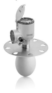
By combining high signal dynamics and FMCW radar technology, this market-entry 24 GHz radar device measures accurately and reliably the level of solids like stone, plastic granulates or coffee beans. No need for expensive antenna aiming kits or purging systems; the proven Drop antenna design minimizes scaling and is not affected by the angle of repose.
