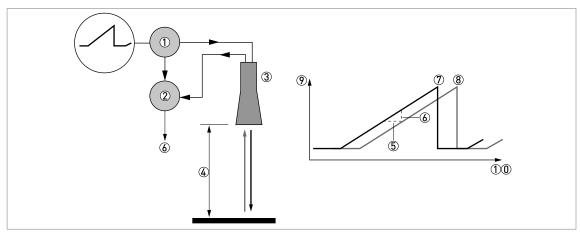
Figure 1-1: Measuring principle of FMCW radar
