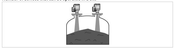
Figure 3-3: There is no maximum limit to the number of devices that can be operated in the same silo
