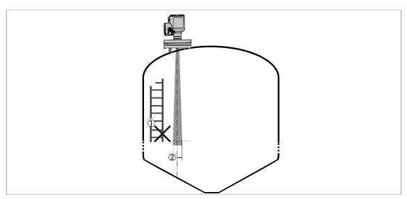
Figure 3-4: Equipment and obstacles: how to prevent measurement of interference signals
