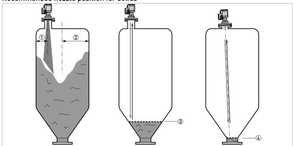
Figure 3-2: Recommended nozzle position for solids
