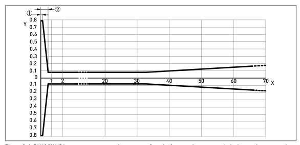
Figure 2-4: DN40 ( $1\frac{1}{2}$ ) Lens antenna: measuring accuracy (graph of measuring accuracy in inches against measuring distance in ft)
