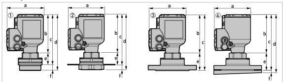
Figure 2-12: DN70 / 3" Lens antenna versions
