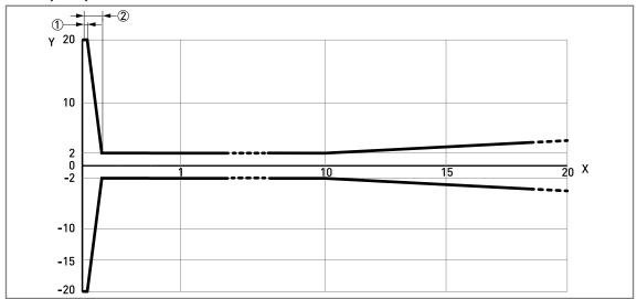
Figure 2-3: DN40 ( $1\frac{1}{2}$ ) Lens antenna: measuring accuracy (graph of measuring accuracy in mm against measuring distance in m)
