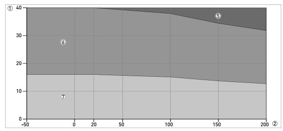
Figure 2-7: Pressure / temperature de-rating (EN 1092-1), flange and threaded connection, in °C and barg
