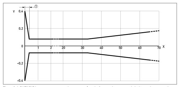
Figure 2-6: DN70 (3") Lens antenna: measuring accuracy (graph of measuring accuracy in inches against measuring distance in ft)
