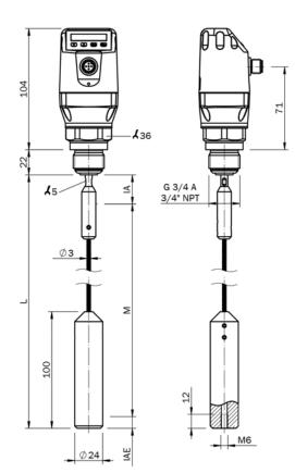
M: Measuring RangeL: Probe LengthIA: Inactive area at process connection: 1 inchIAE: Inactive area at probe end: 0.4 inches
