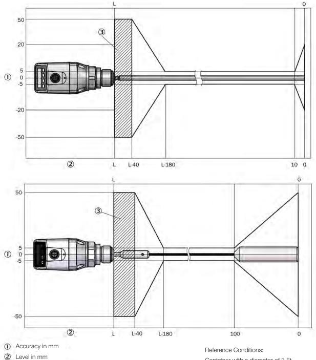
Accuracy Diagram without Parameterized Tank
