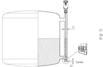
D>= 1.5" Distance tank wall/tank bottom: B >= 0.4"
