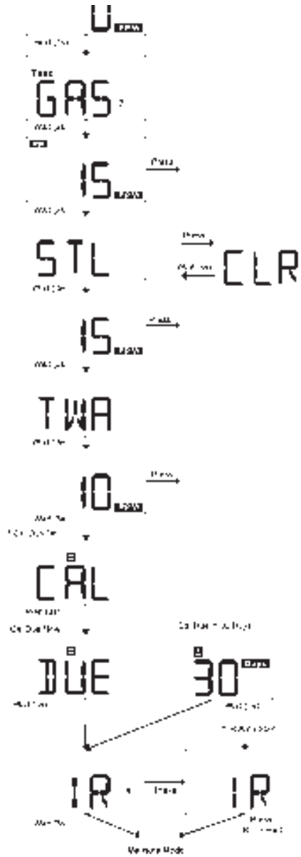
Figure 2-5. Accessing ALTAIR Pro Pages (Does not apply to the Steel Mill Version)
