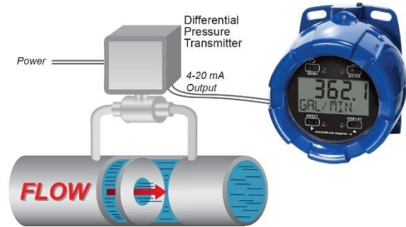
PD6800 Displaying Flow Rate by Extracting Square Root from DP Transmitter Signal.
