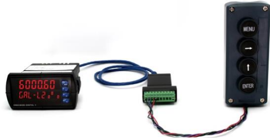
Figure 25. Meter to Control Station Connection
