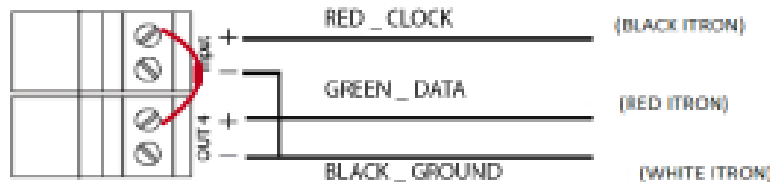
Figure 38: ORION Cellular LTE endpoint connection with resistor
