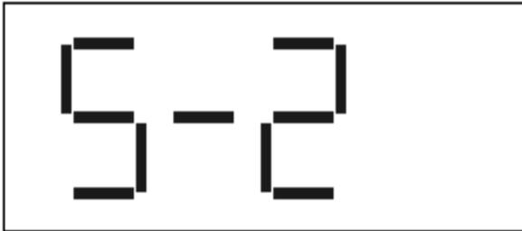
Shown when occur inner failure of transmitter operation occurs, and reverts back to normal condition when the failures are removed.
