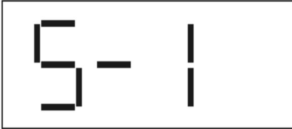
This message present for failures of the sensors such as short circuit, break-down of wire, abnormal wiring, and reverts back to normal condition when the failures are removed.
