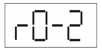
Shown when the target Zero input value is over sensor limit (Minimum Span) in case Span is +, and the input value must be less than sensor limit (Minimum Span)
