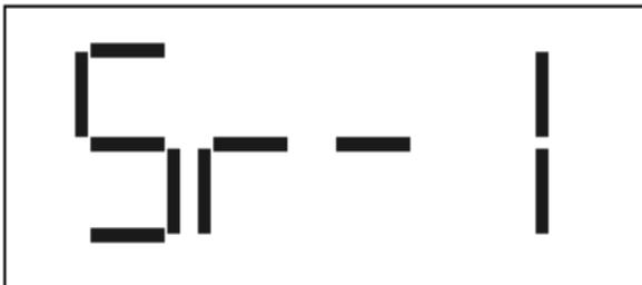
Shown with abnormal sensor type, and reverts back to normal condition when the failures are removed.
