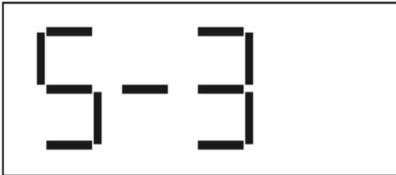
Shown when there is an inner parameter's data error, reverts back to normal condition when the failures are removed.
