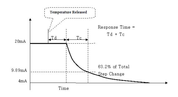
The Meaning of Damping time is to reach 63.2% of target value
