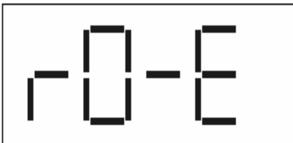
Shown when prohibited writing on EEPROM of inner CPU. In this case, Zero and Span setting is impossible (Permit after EEPROM Writing enable setting)
