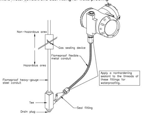
After wiring, impregnate the fitting with a compound to seal tubing.
