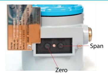
Transmitter's Zero/Span configuration Button
