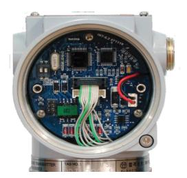
CPU Module Fail Mode, EEPROM-Write Selection Jumper Switch
