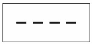
This message will be shown when resetting CPU inner EEPROM Data, and transmitter will be reset when the resetting procedure is done.
