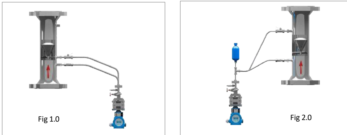
Fig 8: Installation suggestion for upward flowing condition - Cone Meter with Vertical Orientation
