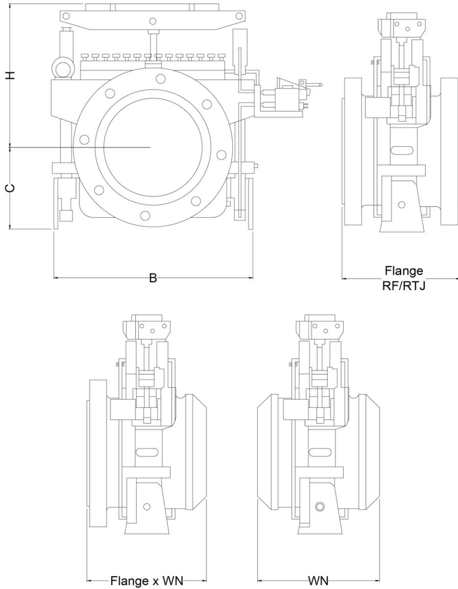
Fig.6. Dual Chamber Orifice Flowmeter
