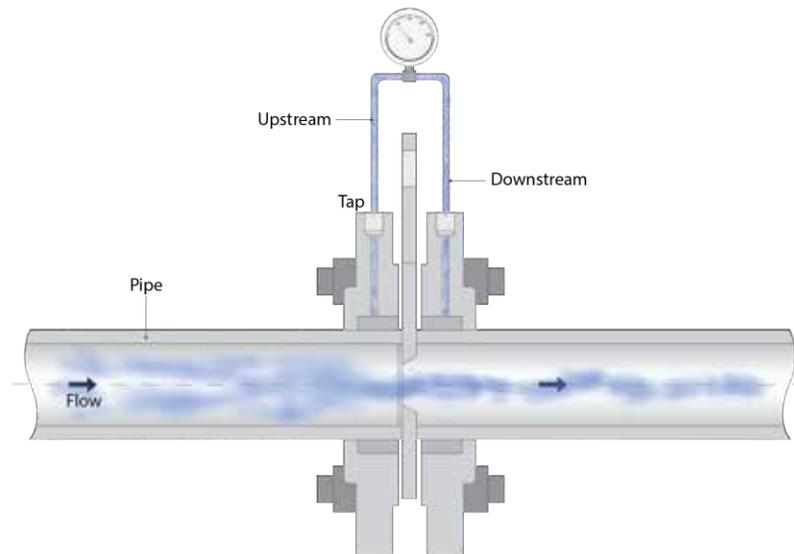
Fig.4. Differential Pressure Measurement
