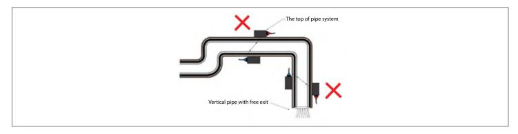
• For the open pipe or half full pipe, the transducers should be installed at the bottom of U pipe.
