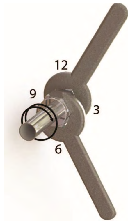
Figure 4 - While holding the fitting's body steady, tighten the nut one and one-quarter turns to the 9 o'clock position.
