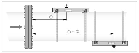
Figure 3-14: Mounting second rail in Z mode (1 traverse) using a reference point
