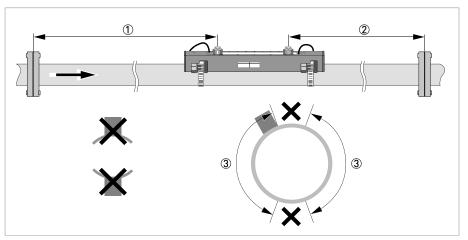
Figure 3-1: Inlet, outlet and recommended mounting area
