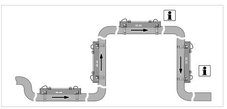
Figure 3-6: Mounting on vertical pipelines is possible
