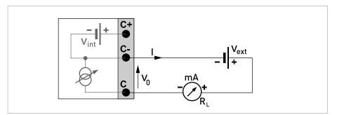
Figure 5-5: Current output passive Ip
