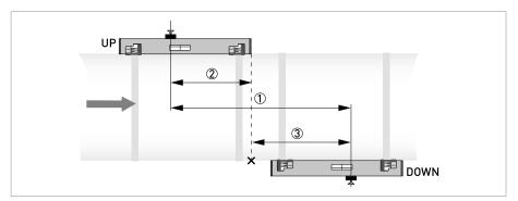
Figure 3-15: Mounting second rail in Z mode (1 traverse) without using a reference point ① Advised distance ① = ② + ③
