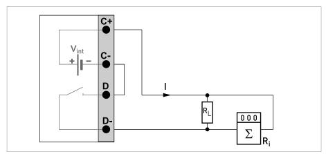
Figure 5-7: Pulse frequency output active P<sub>a</sub>
