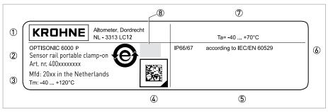
Figure 2-3: Example of a flow sensor nameplate
