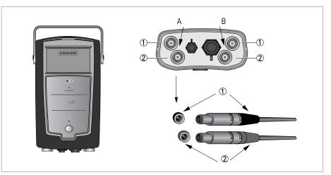
Figure 3-21: Connecting signal cables channel A and B
