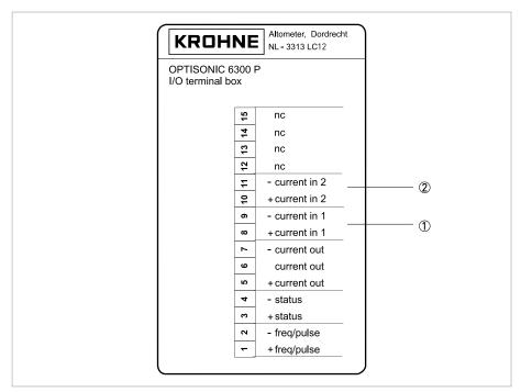
Figure 4-4: Standard I/O box for 4...20 mA temperature transmitters
