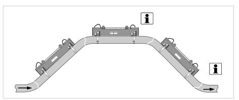
Figure 3-7: Mounting on ascending or decending pipelines is possible
