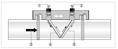
Figure 7-1: Measuring principle (example reflected path set-up)
