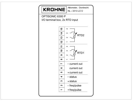
Figure 4-3: Extended I/O box with 2 temperature transmitters included for PT 100 sensors.
