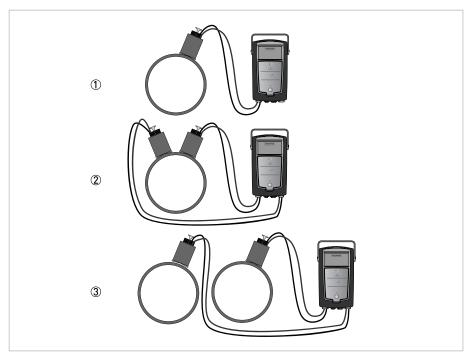
Figure 2-2: System configuration possibilities
