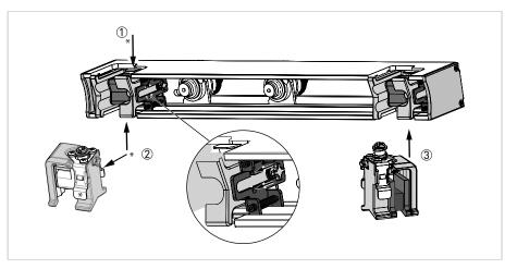
Figure 3-19: Installing magnetic fixation units
