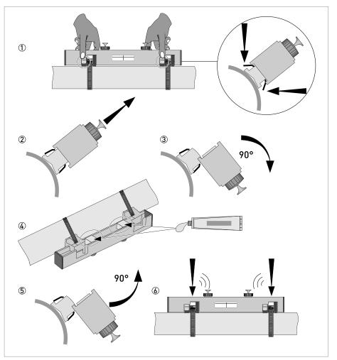
Figure 3-20: Greasing transducers
