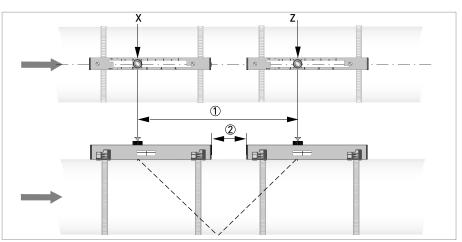
Figure 3-13: Mounting 2 rails in V-mode (2 traverses)
