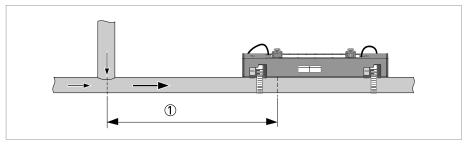
Figure 3-4: Distance behind a T-section (1)  $\geq 20 \text{ DN}$
