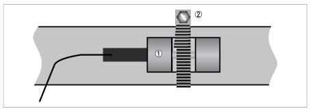
Figure 4-2: Mounting PT 100 with hose clamp
