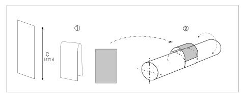
Figure 3-17: Fold paper and place back on pipe line
