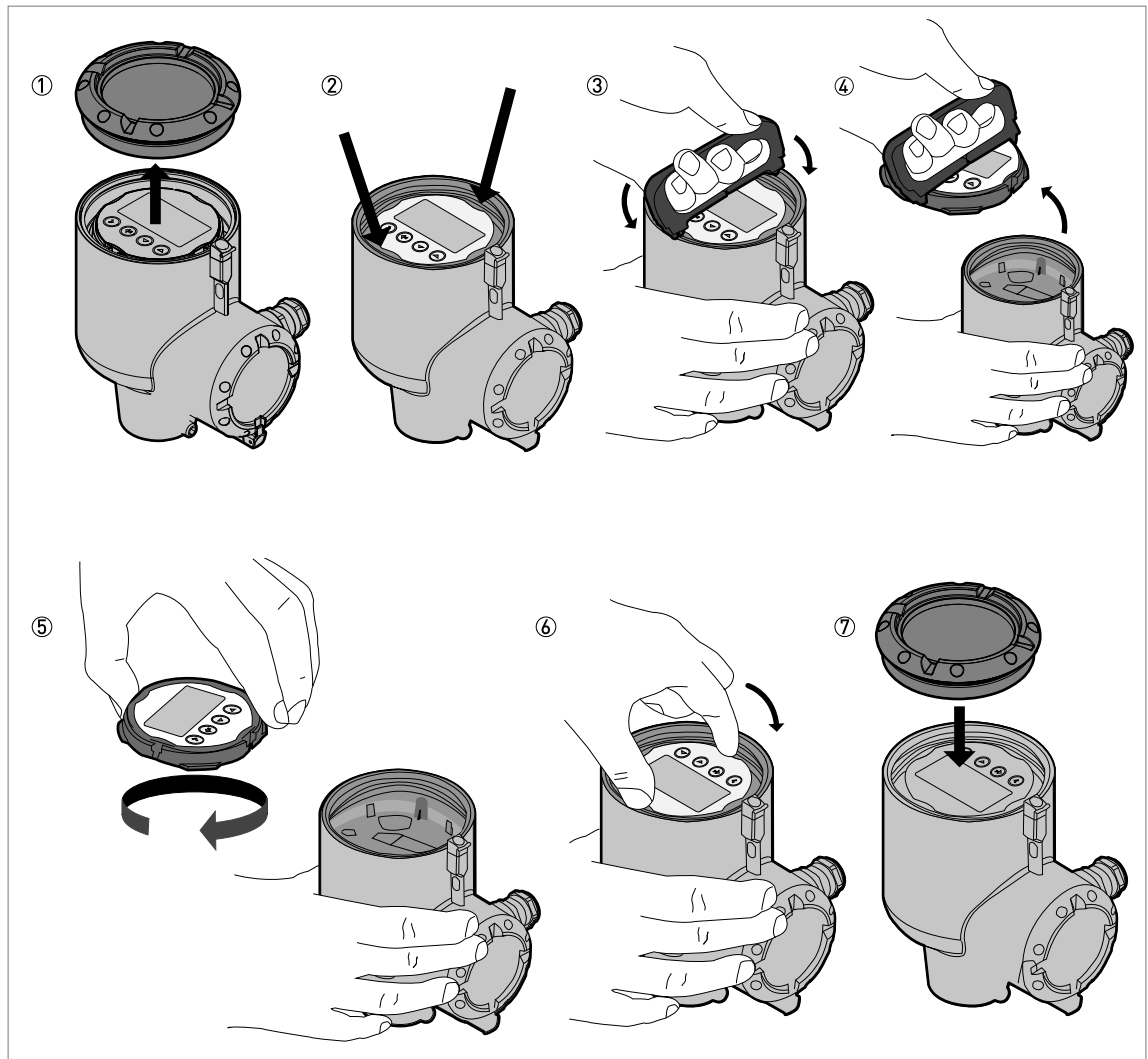
Figure 3-15: How to turn or remove the display module (option)
