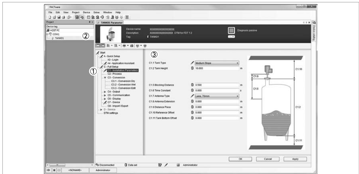
Figure 5-5: Screen from the PACTware™ user interface
