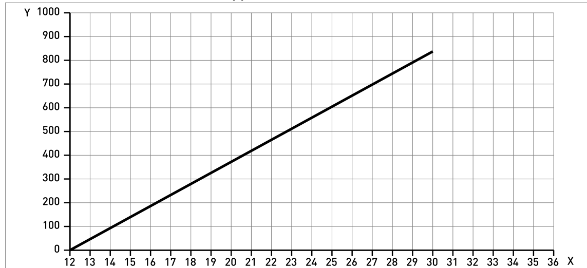
Figure 8-6: Minimum power supply voltage for an output of 21.5 mA at the terminals (Non-Ex and Hazardous Location approval (Ex i / IS))
