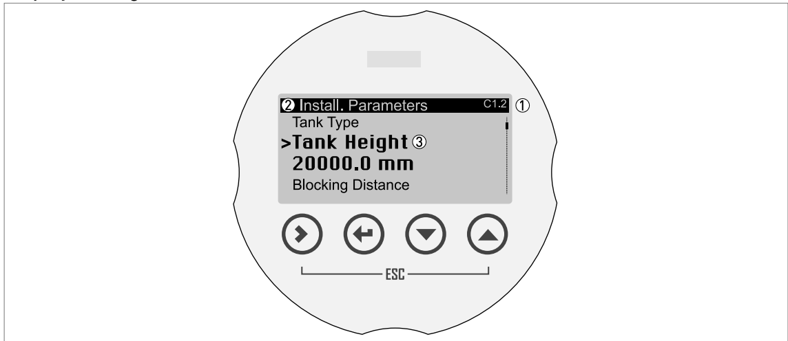
Figure 5-2: Display screen layout in Program mode
