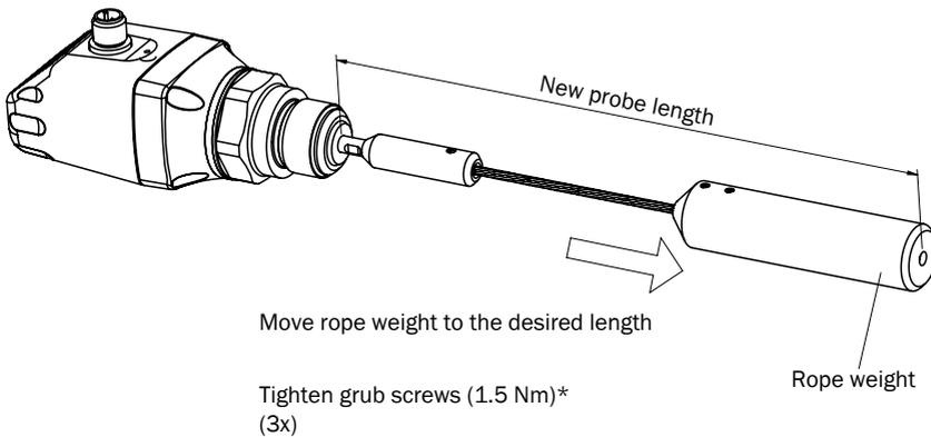
\*We recommend to use thread locking fluid to secure the grub screws
