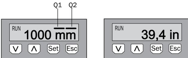
**Note:** The statuses of the switching outputs are indicated in millimeters by bar graphs above the unit. This display is not available when inches are selected as the unit.
