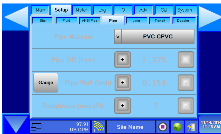
Figure 54: Pipe page from nominal entry
